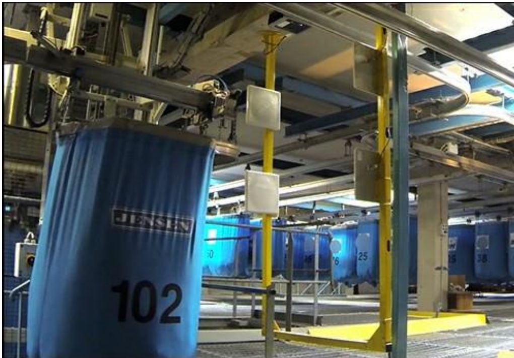
Soiled linens are returned to BIH in large "sling" bags, which are hung on a conveyor and identified as they pass a read area.
