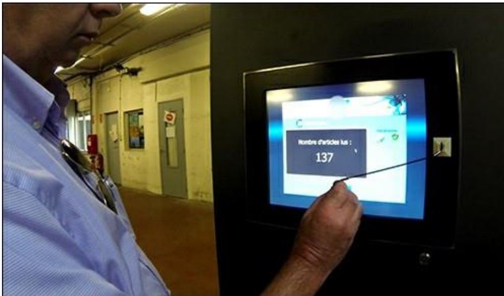
After pushing a clean-linen trolley into the cabin, a worker uses the integrated computer to activate the reader and perform a count.
